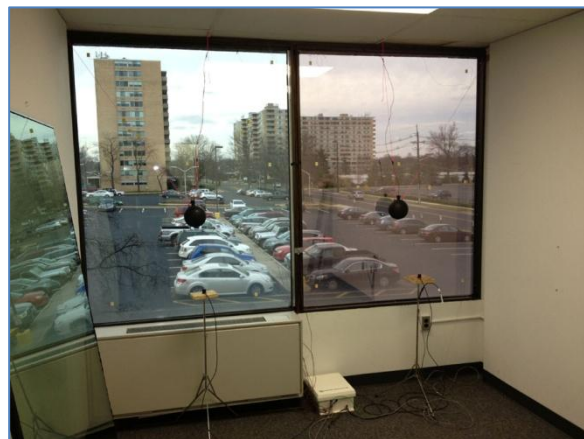
Figure 3. Test Office with One Low-E Retrofit Panel Installed (left side)
